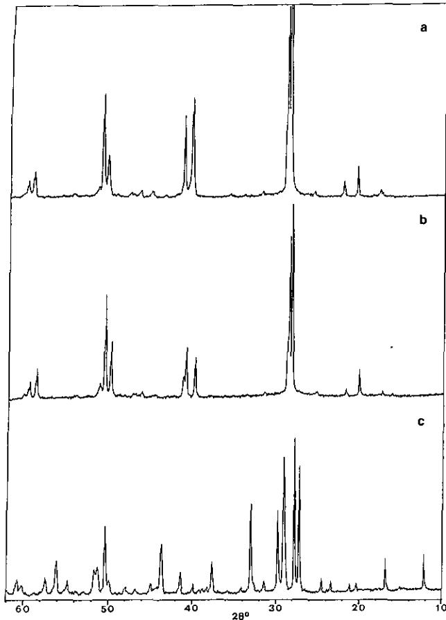
FIG. 7. Room temperature X ray diffraction patterns of \text{BaBiO}_{3-\delta} ( \delta = 0.44 ) annealed in silica glass tubes: (a) at 900°C; (b) at 700°C; (c) at 650°C.
